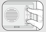
Press and hold both buttons on the new intercom for 5 seconds. An initial beep will be heard followed by a second beep. The channel lights will flash. Within 10 seconds put any networked intercom into Learn Mode (refer to table below).
